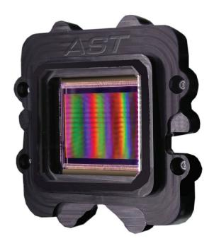
The 27.1 GPixels/s raw throughput rate is the fastest in the industry. No spatial or temporal interpolation. Raw speed, the 168ns shutter time is also among the fastest. We even optimized the 13.5  $\mu$  pixel size for the proper balance between high-resolution (for image clarity) and exceptional light sensitivity normally found only with larger pixels.
